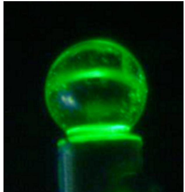
Figure 4 (online color at: www.lpr-journal.org ) Upconversion green image mapping the optical pump WGMs in an erbium-doped phosphate microsphere with a diameter of approximately 150 micrometers.
