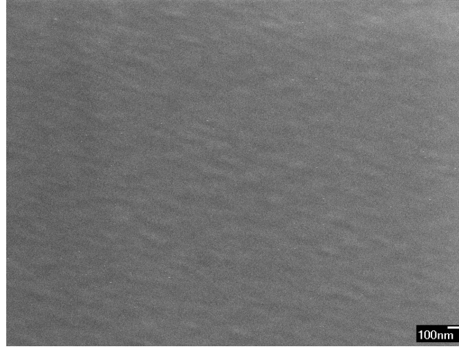
Fig. 24. – SEM image of the surface of a 160 nm thick silicon-rich oxide ( \text{SiO}_x , x \approx 0.3 ) thin film deposited on a silica substrate using the LPCVD method [136]
